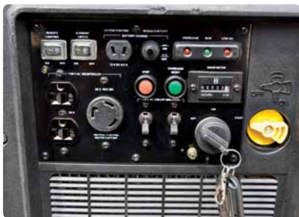
▲ The control panel is nothing out of the norm—a few circuit breakers, switches, electrical plugs, etc. The wireless remote start was the feature we liked the most, partly because it was fun to play with. The ability to control it with a key fob like the one you use to unlock your car means no more getting out of the RV to start or shut off the generator whenever the need arises.
