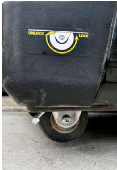
▲ While the Honda has a wheel option, the Powerhouse comes from the factory with a nice set of locking urethane wheels. The wheels combed with the wheelie bar, made transporting this generator a walk in the park.
