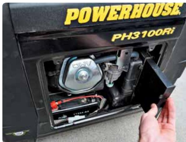
▲ It's important to note that no generator is shipped with oil in the engine's crank case. Many dealers will add the oil for you, but it's of utmost importance to make sure the engine has oil before starting it. We filled ours with 15W-45, as per the manufacturer's instructions.
